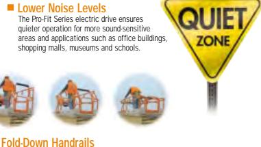
Standard on four models including the compact Model 2030ES which allows access through doorways as low as 71.5 inches (1.82 m).
